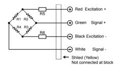
Note: 6 Cores cable is optional. Do not change the length of cable, or lese, it will effect the sensitivity of load cell.
