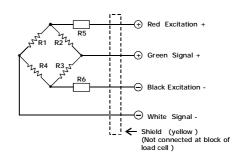
Do not change the length of cable, or lese, it will effect the sensitivity of load cell.
